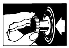
C. Start the washer by pulling out the Control Knob. The washer will fill to its highest level with wash water of the selected temperature. After filling, the washer will agitate for the selected number of minutes.
